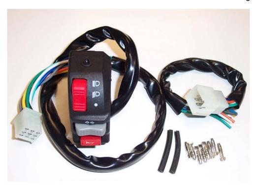
Off-Road Handlebar Switch (K&S Stock # 12-0055CN)
